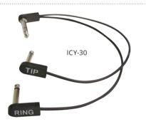
**EBS ICY-30** Insert Cable designed, but not limited, to use with the Billy Sheehan pedals. A stereo (TRS) plug splits into two mono 1/4" plugs, representing the TIP and RING of the TRS plug to create a loop. 30 cm cable length.
