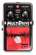
**EBS MultiDrive Studio Edition** is a 'class A' overdrive pedal, capable of producing sustain, overdrive and many other useful 'tube amp' distortion sounds.
