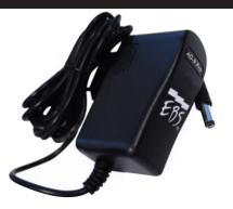
**EBS AD9 Pro** is a 1000 mA, 9V DC power supply that only takes up one outlet spot. It handles everything between 100-240V. Short circuit protected, clean and hum free 9V DC power output. 2.1 mm, center negative contact.
